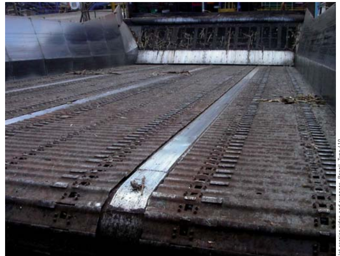
Slit carrier sides and runners, Brazil, Type 410
