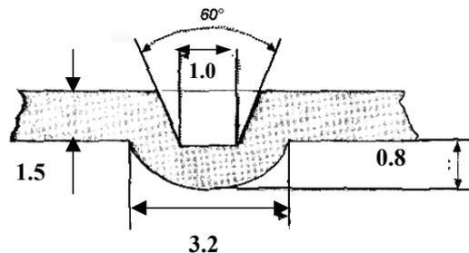
Figure 9 The projection and its dimension in mm.
