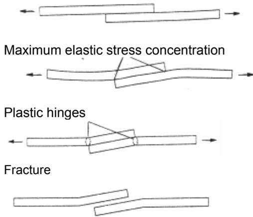
Figure 1 Deformation of lap joint during loading.
