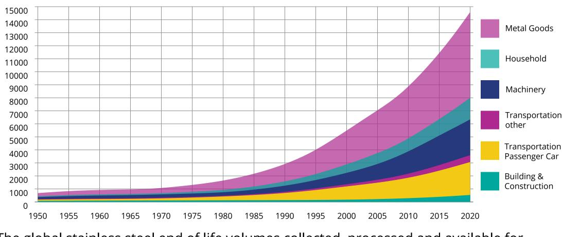
The global stainless steel end of life volumes collected, processed and available for recycling. Scrap is melted and transformed into new sustainable stainless steel products which can in turn be recycled at the end of their life.
