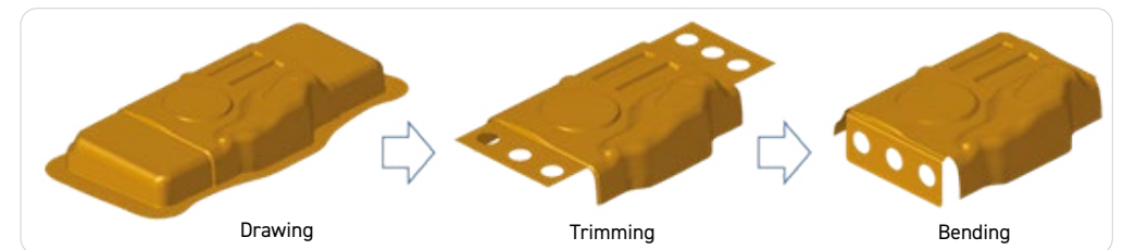
Figure 2 Manufacturing process of baffle integrated part Copyright 2020. POSCO Co., Ltd. All rights reserved.
