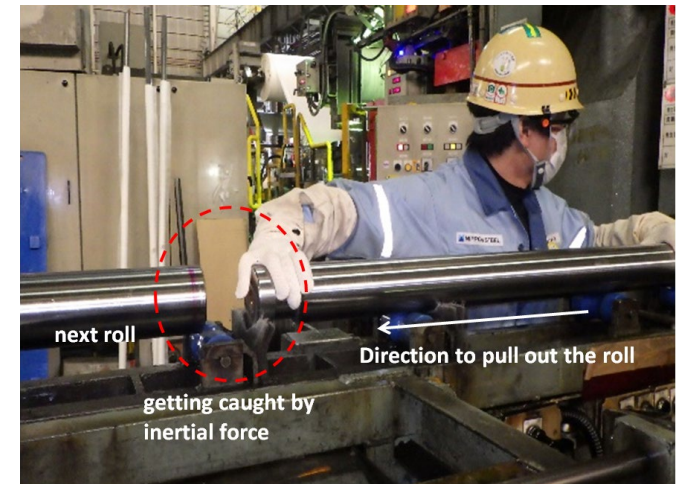
Photo 1 Roll replacement operation for Sendzimir mill
