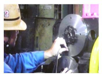
Shear cutting blade exchange
