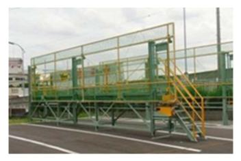
Equipment solution 1 A net is fitted closely so a fall from the track bed will cover the gap can be avoided
