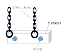
Figure 1: Old lifting device
