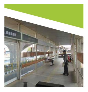
Sixty bus shelters have been installed in Ahmedabad by the Ahmedabad Municipal Corporation. Stainless steel was utilised as it met the Corporation's key requirements for corrosion resistance, durability, crash resistance, fire-safety, ease of cleaning and maintenance, and visual attractiveness.
