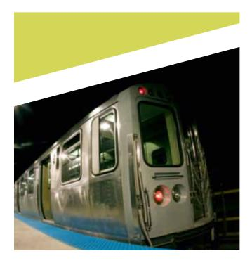
Stainless steel is utilised for these Brazilian subway carriages because of its mechanical and corrosionresistance properties.
