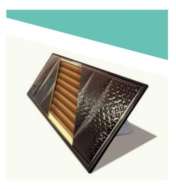
This integrated solar collector has been made with a ferritic grade of stainless steel. The collector produces hot water for domestic consumption. The system is fully autonomous and utilises a recirculation pump powered by photovoltaic (PV) cells. All parts of the system are integrated within the absorber. This includes the 150 litre storage tank and PV recirculation system.
