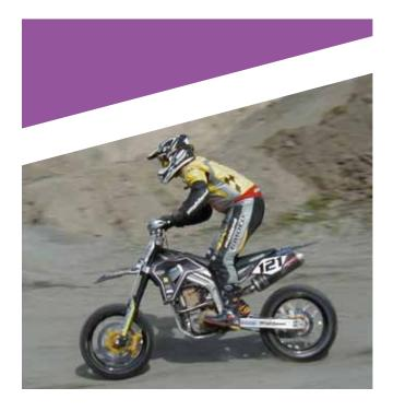
The main frame of the Highland 450cc Supermoto is made from austenitic HyTens1200<sup>®</sup> (1.4310 C1200) while the engine cradle and rear sub-frame are made from duplex LDX 2101<sup>®</sup> (1.4162) box sections.
