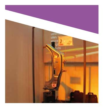
Stainless steel grade AISI 301 can be used for the A-pillar of the body in white (BIW) of production vehicles. The use of AISI 301 will lighten the A-pillar by 1.8 kg (24%) compared to DP 600 carbon steel which has been used in this application until now. AISI 301's high level of formability enables parts integration and shape optimisation for vehicle manufacturers.
