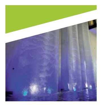
Standing at eight-metres high, this indoor water wall has been constructed from mirror-polished stainless steel mesh. Even with long-term contact with the water, stainless steel will remain free of corrosion and the wall will maintain its beautiful appearance. The stainless will not leach any harmful substances into the water or the environment.
