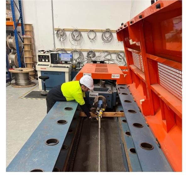
that are characteristic of wire rope. 2205 duplex stainless steel was recommended and ultimately chosen as the material of construction to reduce the risk of pitting and crevice corrosion, in addition to its tensile strength, longevity and life-cycle cost-effectiveness.
