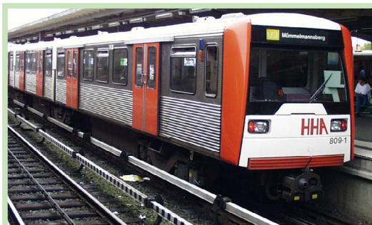
Positive long-term experience with the DT-3 ensured Hamburger Hochbahn opted for stainless steel in its next generation of trains (Photo: Hamburger Hochbahn AG)
