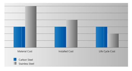
Cost comparison of 0.6 mm coated galvanised carbon steel and 0.4 mm stainless steel grade 1.4401: Due to the mechanical properties of stainless steels, the material thickness can be reduced to 0.5 or 0.4 mm, providing a lighter weight (3.2 kg/m<sup>2</sup> for 0.4 mm stainless steel as against 4.7 kg/m<sup>2</sup> for 0.7 mm coated carbon steel). While coated carbon steel has a life expectation of 15 to 20 years, the service life of a stainless steel roof is generally that of the building.
