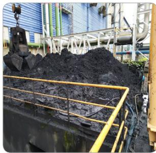
*Metal Scale generated from Scale Breaker*
