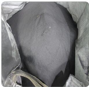
*Metal Oxide Dust generated by Acid Regeneration*
