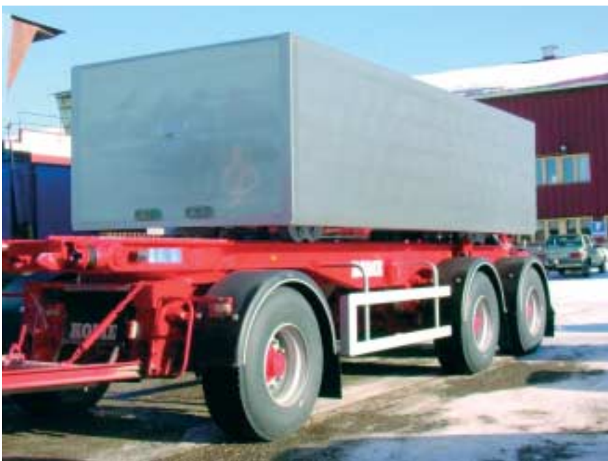
Figure 5. In the special container for gravel truck the stainless steel sandwich panels as side walls are welded to wear resistant plates in the bottom of the structure. A Mo-alloyed stainless steel grade 1.4432 (AISI 316L) has been used. (Photo: Kennotech Oy)
