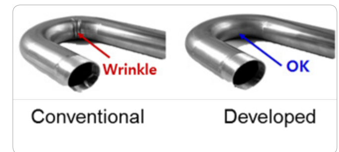
Figure 2: Pipe bending with conventional and developed ferritic stainless steels Picture courtesy of POSCO
