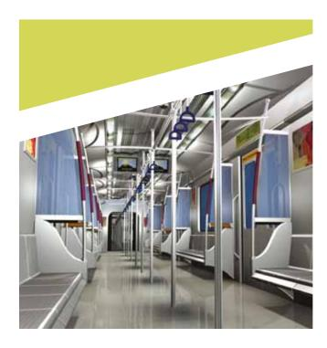
Developed for the New Delhi metro, this railcar features a high-quality, and comfortable, stainless steel interior. The manufacturer specified stainless steel for its fire resistance, light weight and good resistance to corrosion. Another consideration was that the surface of the stainless steel does not require any coatings, further reducing maintenance and running costs.
