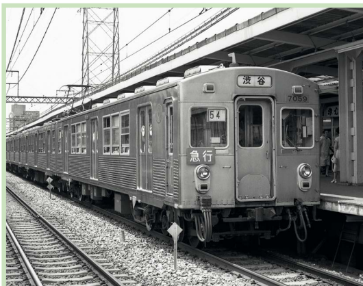
Japan's first all-stainless steel railcar (Tokyu's 7000-series) (Photo: Tokyu Car Corporation)
