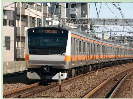
Recent stainless steel commuter train (JR East Japan's E233) (Photo: Tokyu Car Corporation)
