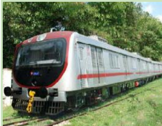
Unpainted metro-car in Austenitic Stainless Steel (Photo: Indian Stainless Steel Development Association)
