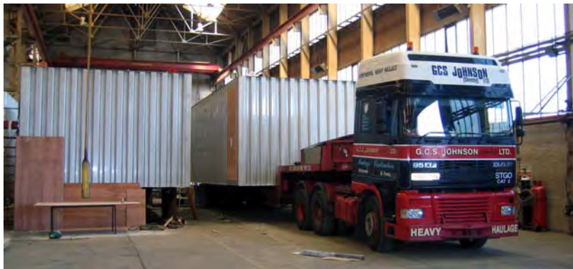
Figure 8: Accommodation module ready for transporting
