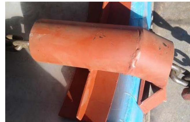
*Steel coil edge protectors have reduced the damage to coils by chains.*
