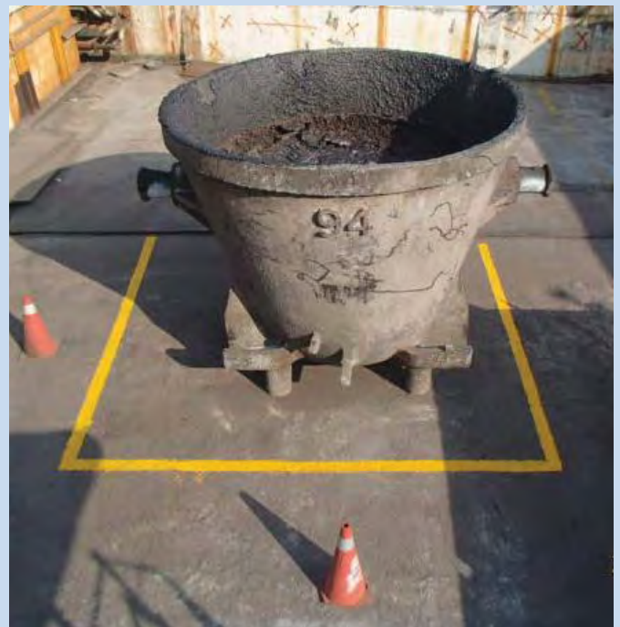
The slag pot cannot be filled above the cylindrical protrusion which is used to tip the pot
