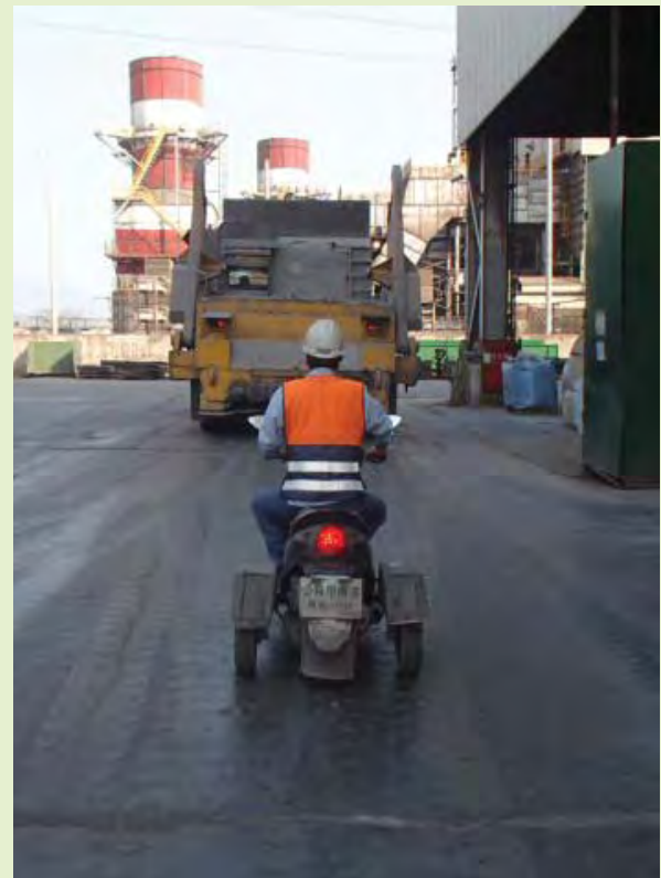
A safety person rides behind the slag-pot vehicle during transportation
