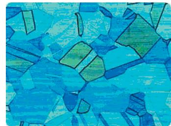
The austenitic microstructure of stainless steel
