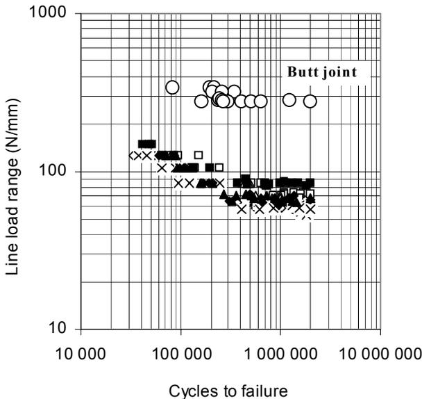
Figure 32 Fatigue properties of laser welded lap joints.
