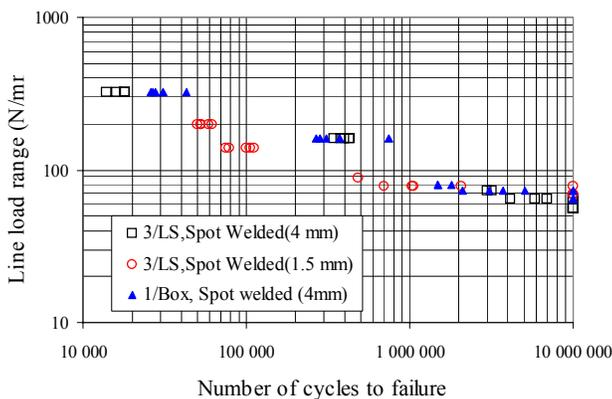
Figure 4 Fatigue properties of spot welded AISI 304CS.
