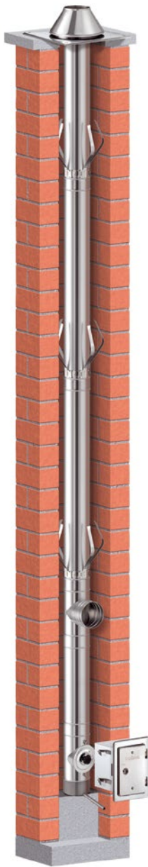
Rigid liners reduce the diameter of pre-existing chimneys, optimising draught and preventing unwanted condensation. Photo: Schiedel, Vienna (A)
