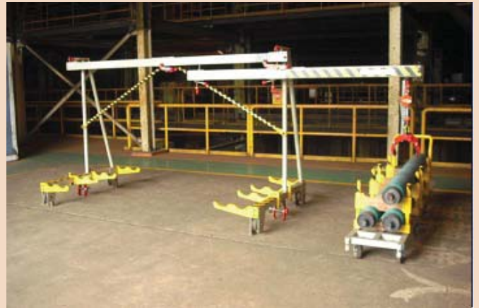
The new roll-change equipment
