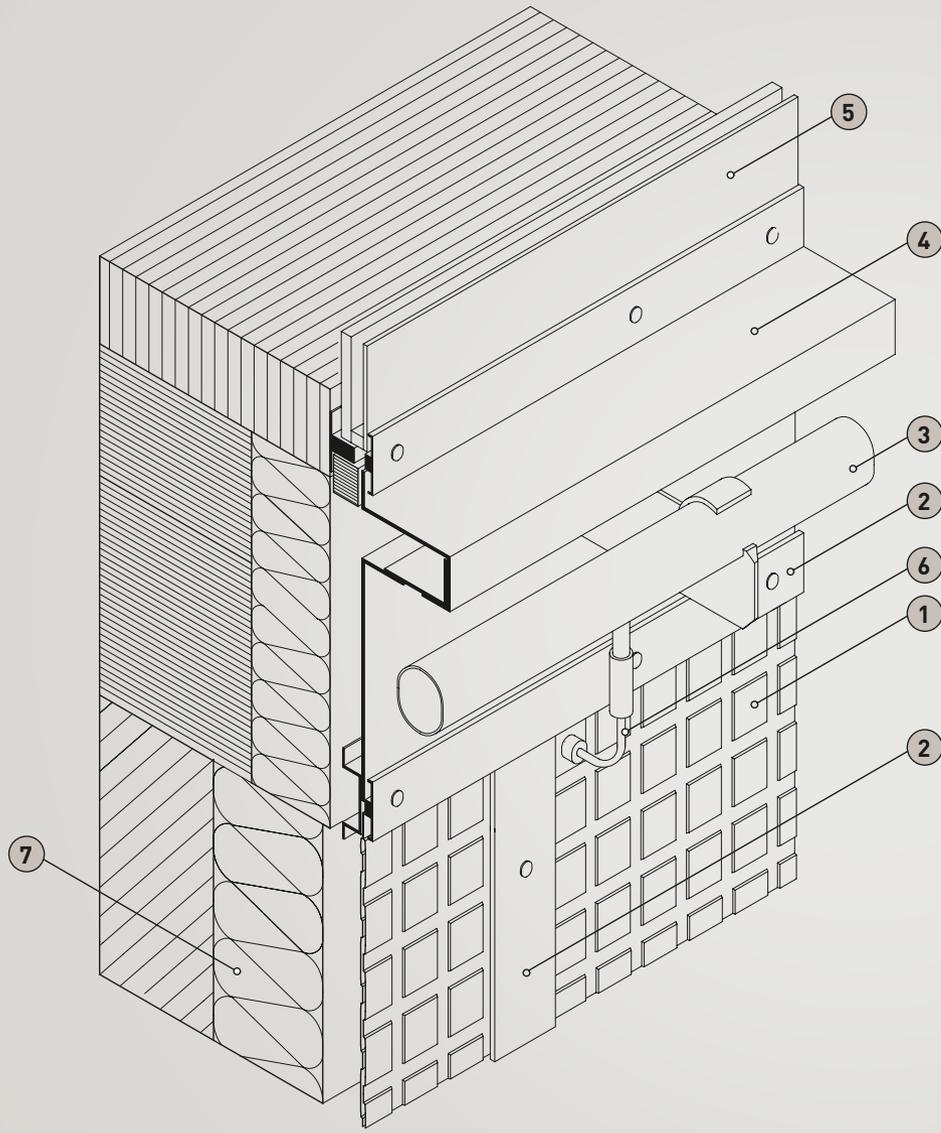
**FIGURE 10:** Detailed view of upper connection of solar collectors to the windows on the upper floor:
