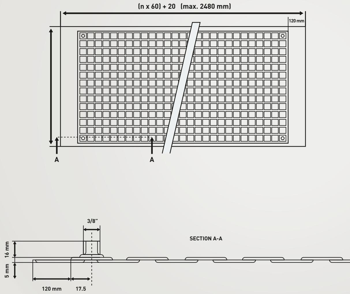
**FIGURE 1:** The principle of stainless steel cushion panels: two patterned, black-chromed stainless steel sheets are assembled back to back. The peaks and troughs are shifted against each other so the fluid can flow through the resulting voids. In contrast to conventional panels, the fluid is in contact with nearly the full surface of the absorber sheet. This principle makes the heat transfer particularly efficient.
