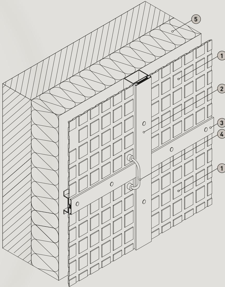
Collector panels are fixed using aluminium profiles with EPDM<sup>1</sup> joints. The profiles are used to fix conventional metal cladding. Once mounted, the facade is watertight and durable.
