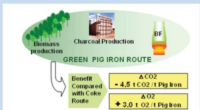
Theoretical CO<sub>2</sub> and O<sub>2</sub> Balance in Pig Iron Production
